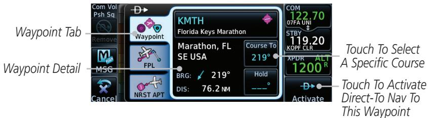
Figure 5-5 Selected Direct-To Flight Plan Leg
