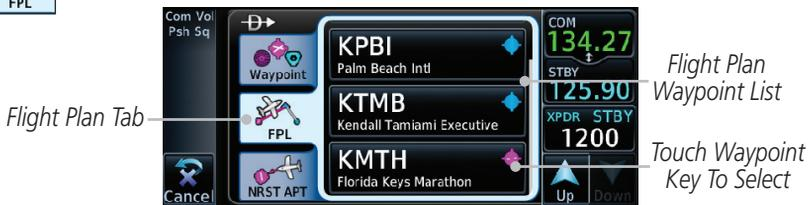
Figure 5-4 Direct-To Flight Plan Leg Selection
