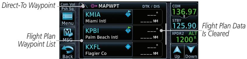
Figure 5-10 Active Flight Data is Removed When a Direct-To Course is Activated
